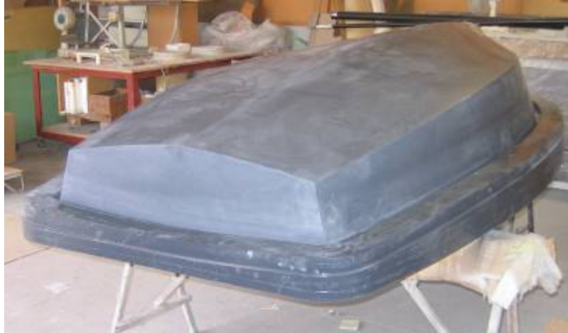
The new Townson/Clinton dimensioned solid MDF Starling plug during final preparation, prior to mould construction.
